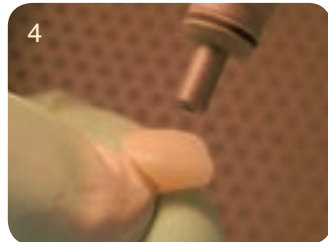
Perform Almina sandblast on the surface of the unpolished area of the crown (50~70μm, 30psi)
