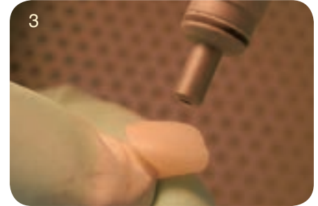
3 Alumina sandblast surface of the crown (50~70µm, 30psi, 0.2MPa)
